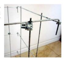
**Step 10:** Lay the base cage on a flat surface. Next, feed the extension cage legs over (outside) the top rim of the base cage. Slide the Wire Rope Clips to clamp the two cages together on the 4 rails. It is not necessary to attach wire rope clips to all 12 legs, but if you have extra clips, attach additional ones as you desire.
