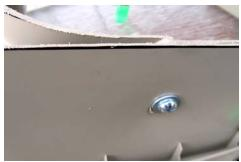
Invert the Support assembly and place into the Container #1 (handles facing up), making sure that you have the lid cut-out properly in place inside the container first.
