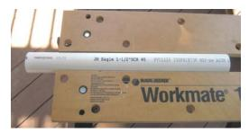
Approximately 1" up from the bottom, drill two 3/8" diameter holes through both sides of the pipe. Move up another inch and repeat drilling another 2 holes.
