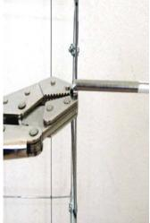
Consistency is most important in making the 3 bends. The goal is to get each 90 degree bend such that the mark falls on the inner or outer radius. The tighter the "fit" of the Tube to the cage, the sharper the bend that can be made at each mark.
