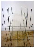
**Step 9:** Place Wire Rope Clips on the 4 vertical rails on the outer top sides of the base cage. (These will loosely sit on the 4 vertical legs at the top rung for the moment. They will be slid to the top of the rails for anchoring the extension cage.)
