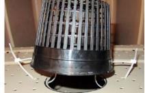
Pull the zip ties tight so the wicking basket is secured over the center of the opening. Cut off excess.
