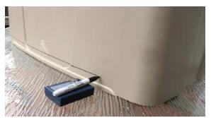
**Step 13:** Secure the Aeration Bench in a Work-Mate or firmly grasp the edge, then cut off this 1-3/8 inch section. NOTE: Use manual tin snips or kitchen shears for this Step.
