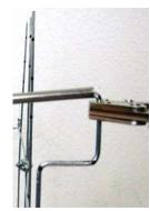
This it the final shape you want after the three bends have been made. Note that the radius of each bend aligns with the marks.
